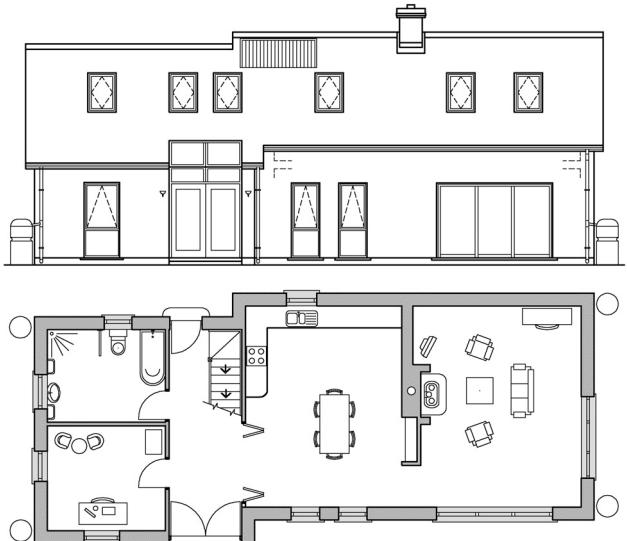
7. A chimney is designed to accommodate a modern wood-burning stove, as shown in the accompanying sketch. The chimney is located on an internal 215 mm solid concrete block wall between the living room and the kitchen. The flue from the stove to the main flue liner is 150 mm in diameter. The floor is an insulated solid concrete ground floor with a 20 mm floating hardwood finish. The dimensions of the stove are: height 700 mm, width 550 mm, depth 450 mm.
